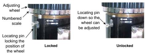
The grind adjustment wheel is held in position by a locating pin. Hold the pin down to move the wheel.
