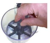
Adjusting the dose of coffee dispensed with each pull of the dosing lever
