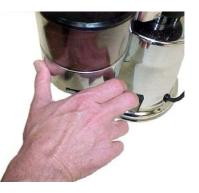
It's important when adjusting the dosing quantity to *roll the coffee*. This is done by placing the dispenser lid under the dosing unit outlet and operating the dosing lever so coffee grounds fall onto the lid. Do this about five times then return the ground coffee on the lid back into the dispensing unit. Repeat this process once more to ensure all six dosing chambers have been evenly filled.
