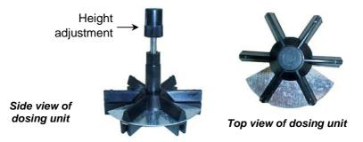
When the dosing lever is operated, the dosing wheel rotates over an outlet that allows the contents of a dosing chamber to be dispensed into the coffee handle/filter basket. This is shown below, in which the dosing unit has been removed from the dispenser.
