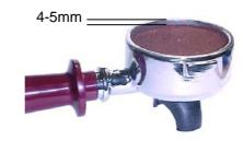
After tamping, the coffee grounds should be around 4-5mm from the top of the filter basket.
