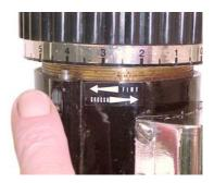
2. Release the adjustment wheel locking pin which will click and lock back into its new position.
